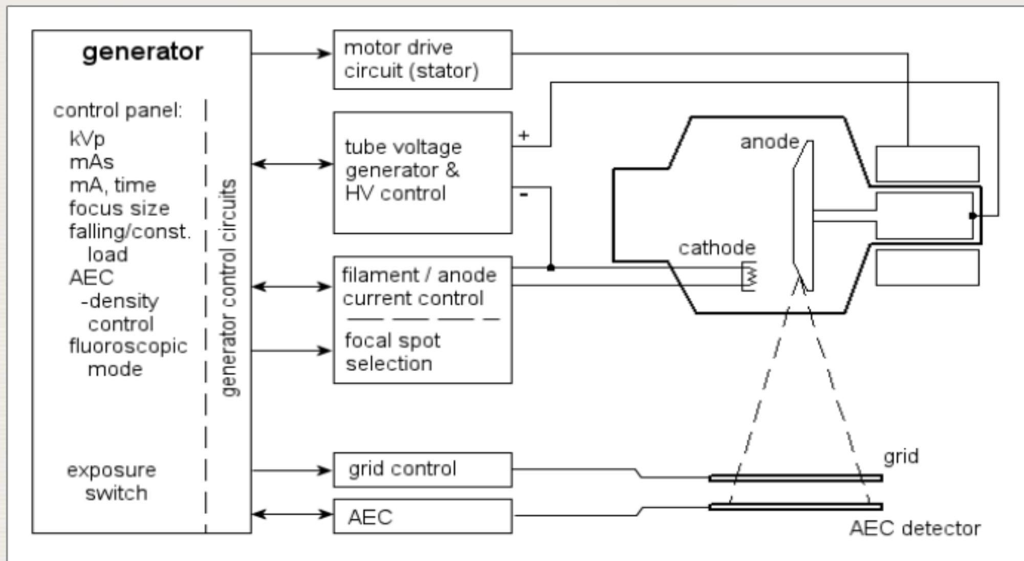
Schematic diagram of a basic X ray generator
