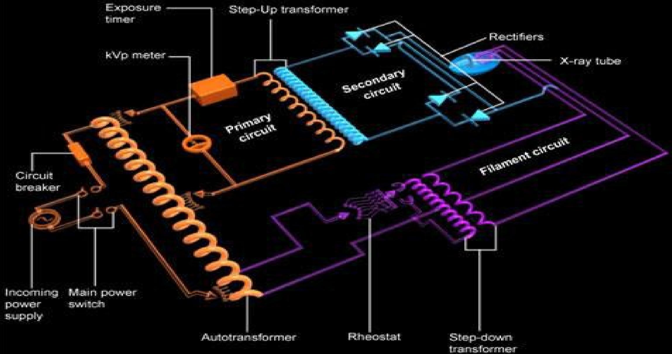
The main circuit and filament circuit are combined to form the complete basic x-ray circuit that is composed of sequence of devices to produce x-rays.
