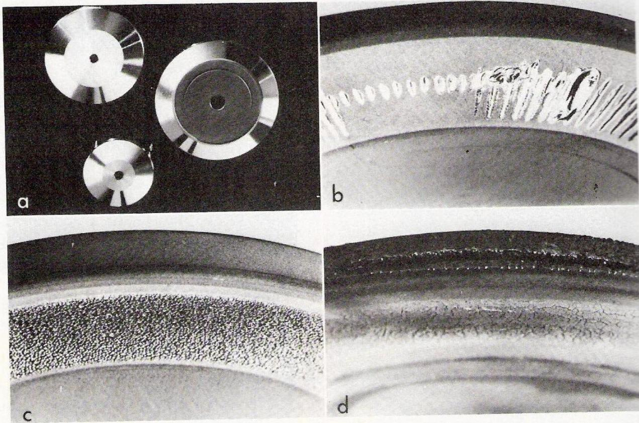
**FIGURE 10-14** Comparison of smooth, shiny appearances of rotating anodes when new, **A**, and their appearance after failure, **B** to **D**. Examples of anode separation and surface melting shown were caused by slow rotation caused by bearing damage (**B**), repeated overload (**C**), and exceeding of maximum heat storage capacity (**D**). (Courtesy The Machlett Laboratories.)
