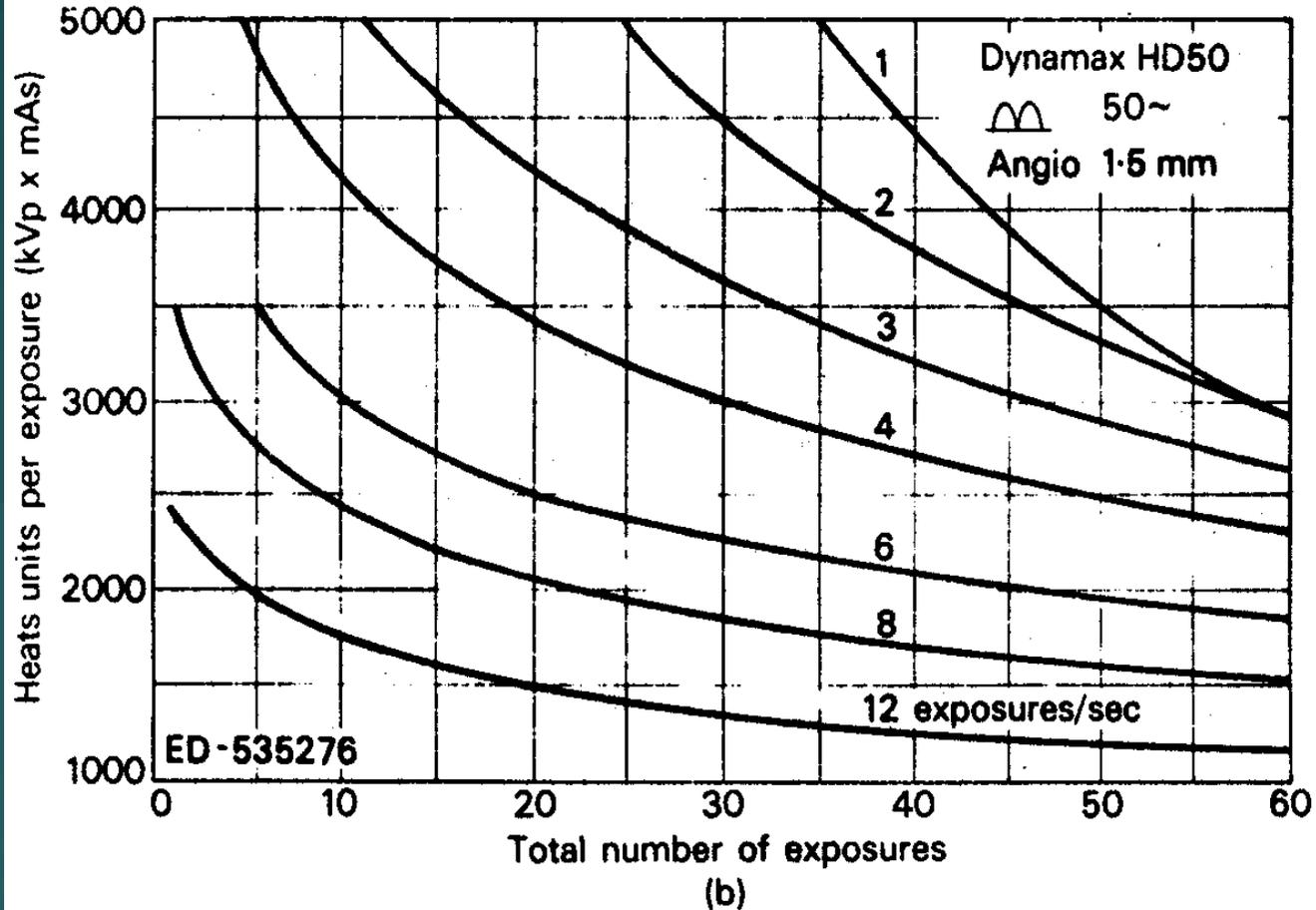
**An exposure factors of 100 kV, 300 mA and 0.05 sec generate 1500 HU**
